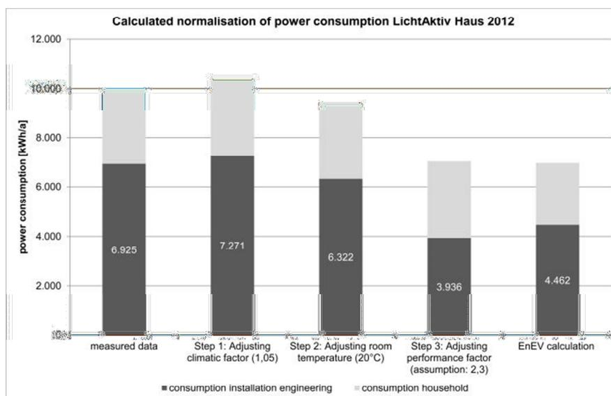
of the system equipment and the original calculations made in accordance with compliance tool submitted, a visual step-by-step tool has been used to follow the steps (fig 4.).
