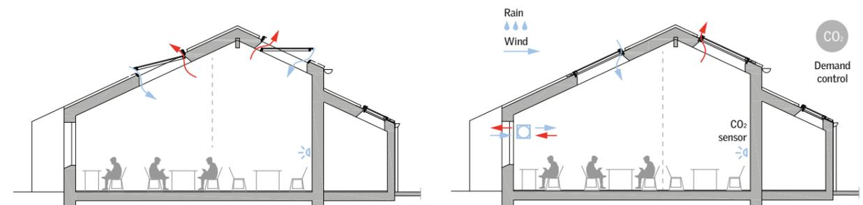
CO<sub>2</sub> sensors control the air quality in the classroom. The roof windows open automatically and close again when minimum CO<sub>2</sub> setpoint is achieved or if it rains.
