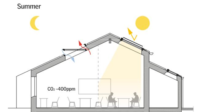
In summer, automatically controled exterior sunscreening helps to control solar heat gains. While manual control of interior blinds provides the possibility of adjusting daylight levels according to the need of teacher and pupils.
