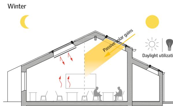
Automatically controlled interior suncreening help to minimise heat losses at night during winter.
